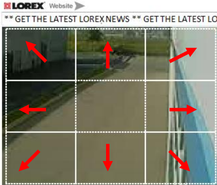
Figure 11: Click and hold the direction on screen you wish to pan or tilt.
