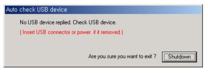
Then, after clicking 'Shutdown' and connecting the USB cable or power cable correctly, you should start the QDU470 server system again.
