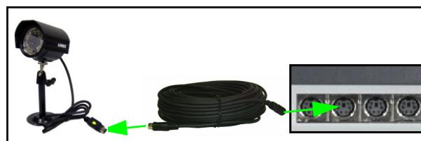
Figure 3.0 Connect the extension cable
