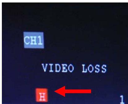
Figure 4. Hard drive detection error, indicated by the red "H" box.
