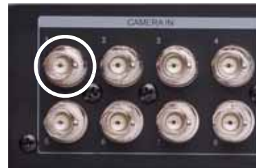
Figure 1.0 Connect BNC cameras to the system
