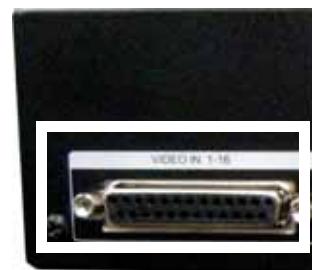
Figure 1.1 Octopus cable port (16-channel only)
