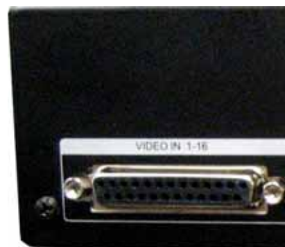
Figure 1.8 Octopus cable VIDEO IN (16-channel only)
