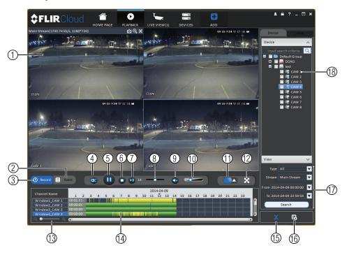
Display area: Double-click to expand/return to split-screen mode. Hold the mouse over the display area to open the camera toolbar.
