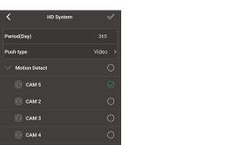
Tap Motion Detect and then check each channel you would like to receive push notifications from.
