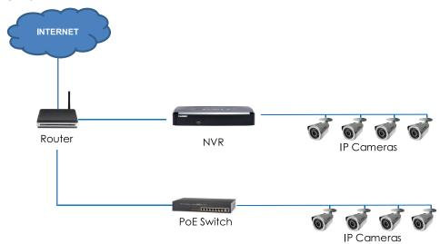
Connect an Ethernet cable from the LAN port on an external PoE switch (sold separately on <a href="www.lorextechnology.com">www.lorextechnology.com</a>) to your router using a CAT5e or higher Ethernet cable. Connect the power cable to the PoE swtich and to a power outlet or surge protector.
