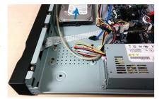
5. Turn the system over carefully. Tighten the hard drive screws (4x) to secure the hard drive.
