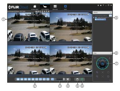
1. **Live display**: Double-click to expand the area. Right-click to access additional options. Hold the mouse over the display area to access the camera toolbar.
