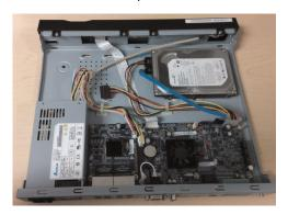
5. Carefully turn the system over. Slide the hard drive and then lift it out of the system.
